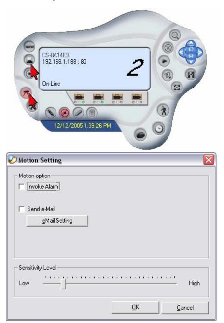
**Step 5** Once the unit is set to the desired configuration you can start recording by clicking on the **Motion Recording** button.
