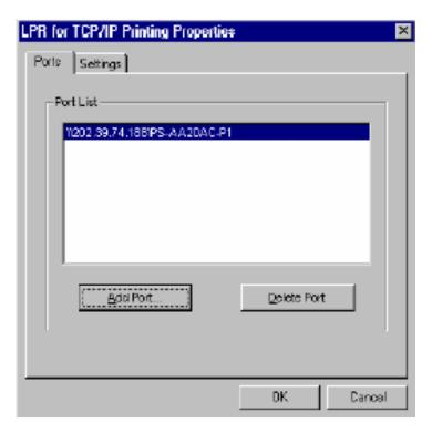
In the top field type in the IP address of your print server. In the bottom field type in the port name of your print server, the Port Name is the PS-xxxxxx-P1, x being the actual number listed in the Port Name box. Click on  $\mathbf{OK}$
