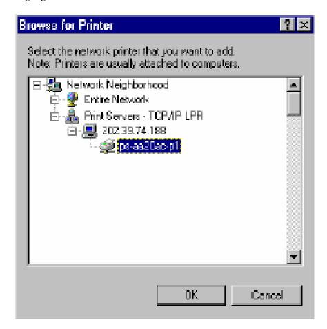
Click on **Next**. If you are unable to do this you can manually enter the Print Server by using two backlashes, the IP address, one backlash and the port name of you printer.
