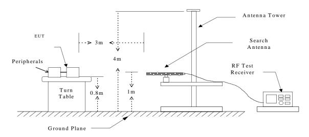
Figure 1 : Frequencies measured below 1 GHz configuration
