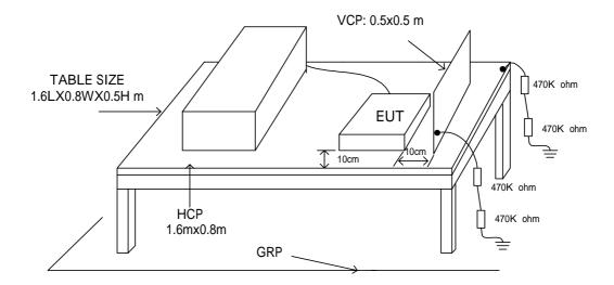
The test setup consists of the test generator, EUT and auxiliary instrumentation necessary to perform DIRECT and INDIRECT application of discharges to the EUT as applicable, in the follow manner:
