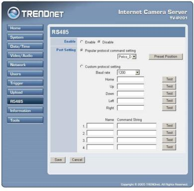
Check the **Enable** item to enable the function of your camera, and configure the related settings in the following fields.
