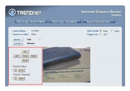
You can use the *Up*, *Down*, *Left*, and *Right* buttons to move the camera's lens to your desired position. Click the *Home* button to return to the default home position.
