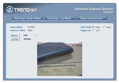
**Camera Name/Location:** The Camera name and location will be displayed when the Camera Name/Location fields are entered in the Web Configuration Utility.
