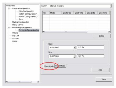
Date Mode: First, select the camera desired from the pull-down menu. Then, setup the time in the Start/Stop fields.
