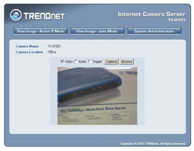
**Camera Name/Location:** The Camera name and location will be displayed when the Camera Name/Location fields are entered in the Web Configuration Utility.
