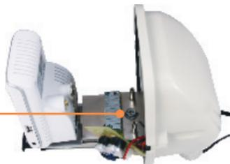
**23.** Screw the circuit board back to the metal bracket.
