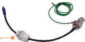
6. Insert the TEW-ASAK through the hole. Then screw in the cap securely.
