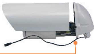
3. Unscrew the circuit board from the metal bracket. Save these screws. You will need to use these screws later.
