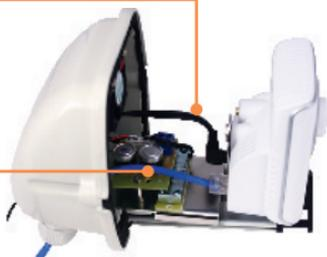
**25.** Connect the Ethernet cable to the Internet Camera server.
