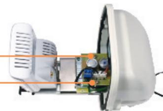
9. Screw the circuit board back to the metal bracket.
