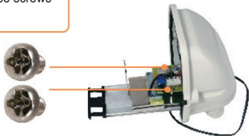
4. Unscrew the metal bracket from the TV-H110. Save this screw. You will need to use this screw later.
