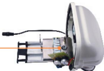
5. Use the following screw to mount the Internet Camera Server to the metal bracket.
