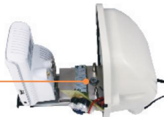
8. Screw the metal bracket back in to the Internet Camera Server.
