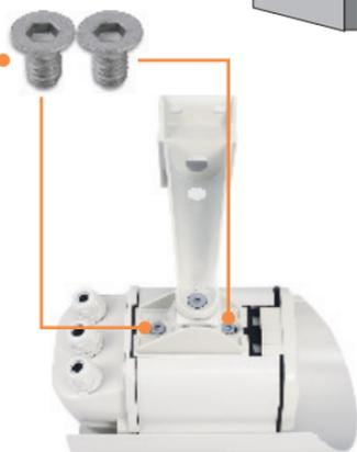
5. Adjust the mounting bracket to the desired position. Then use the provided Allen wrench and turn it clockwise to secure position.
