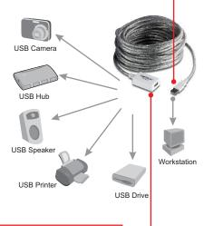
**3.** Plug a USB peripheral device into the USB Type A Female Connector on the TU2-EX12.
