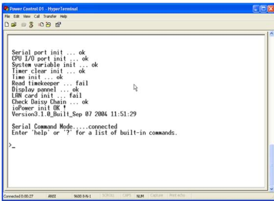
⚡ If the firmware version is lower than 040421, here you should type in `/ TK-RP08 \` on the command line and then hit *Enter* to go into command mode.
