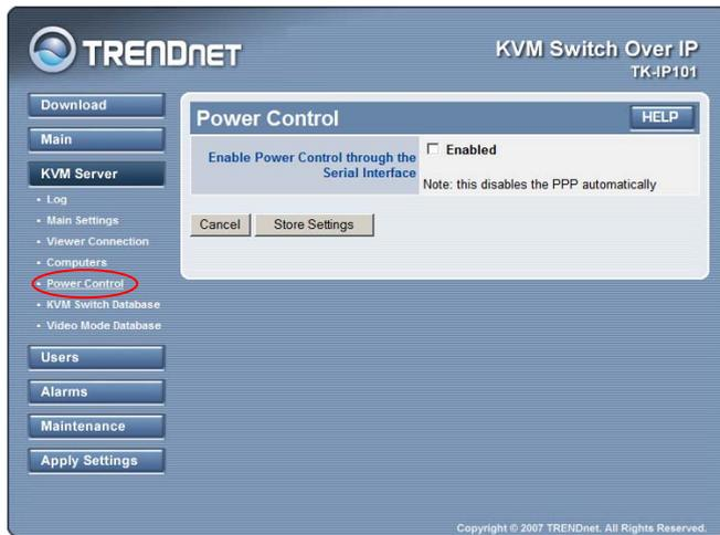
Step 5. Check the *Enabled* option to activate the remote power control support feature of the back panel serial port of the TK-IP101.
