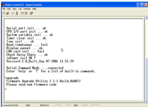
**Step 6.** Type *Upgrade* on the command line and hit *Enter*...Now you have your HyperTerminal ready for file transfer. Keep your HyperTerminal window open and go to the next step....
