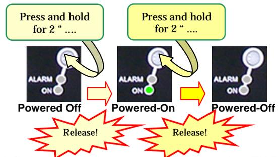
By default, each port is in powered-off state when TK-RP08 is powered on.
