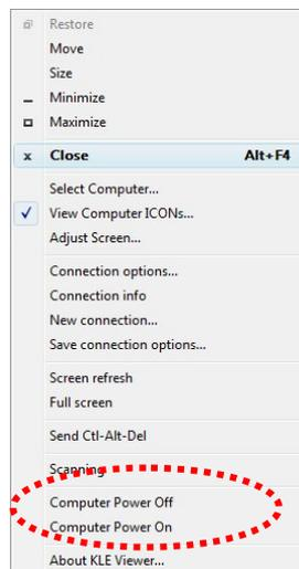
Now you can use the Viewe Quick Menu to perform power on / power off command remotely across internet by using the TK-IP101 together with an TK-RP08.
