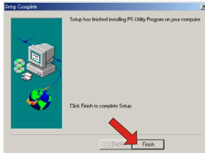
After installing the utility, the application program for the print server is automatically installed to your computer, and creates a folder in **Start\Programs\PS-Utility**.
