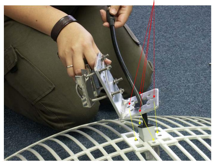
3. Take out the <u>screw</u> from the top of the Feeder's pole, place the <u>Reflector</u> on the pole, place and tighten the screw to secure the Reflector on the tip of the pole.
