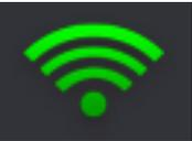
**Wireless:** The wireless icon displays green to indicate that wireless is enabled on both 2.4GHz and 5GHz bands. The wireless icon displays orange to indicate that only wireless band is enabled (2.4GHz or 5GHz). The wireless icon will display red to indicate that wireless is disabled on both 2.4GHz and 5GHz bands.
