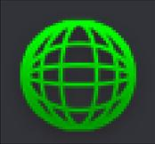
**Internet:** The Internet icon displays green to indicate that your router has successfully established an Internet connection. The Internet icon displays orange to indicate that a physical connection has been established on the Internet port of the router but with no successful Internet connection has been established. The Internet icon displays red to indicate that the Internet is physically disconnected.
