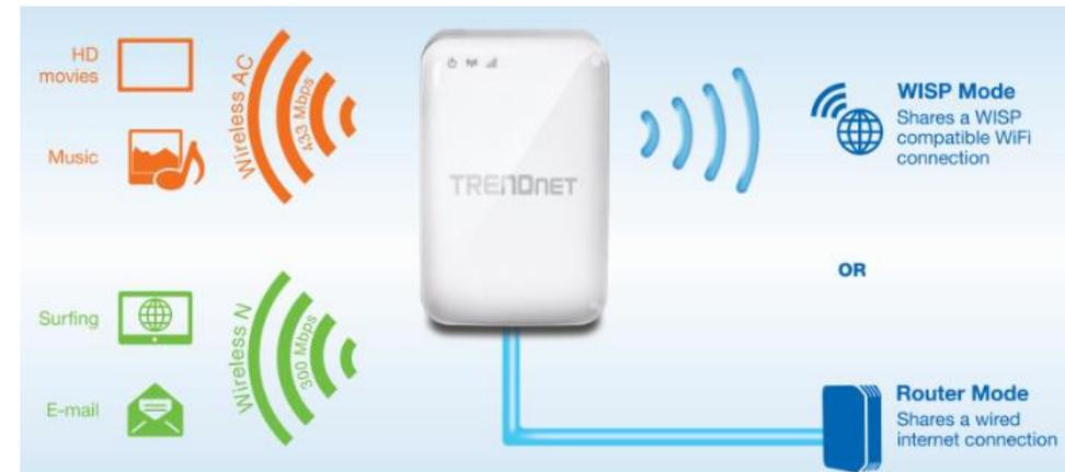
The router is installed near the hotel's internet connection port which connects to the Internet. 2.4GHz wireless signals from the router are broadcasted to wireless clients such as laptops (with wireless capability) and the less congested 5GHz wireless signals from the router are broadcasted to other wireless client devices such as TVs, game consoles, or media bridges thereby providing Internet access for all wireless client devices.
