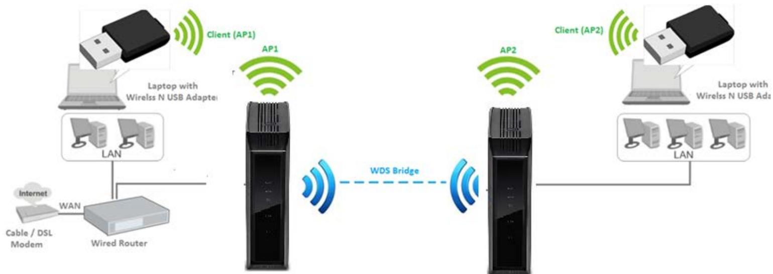
The diagram below illustrates an example of multiple WDS wireless bridge links with access point functionality.
