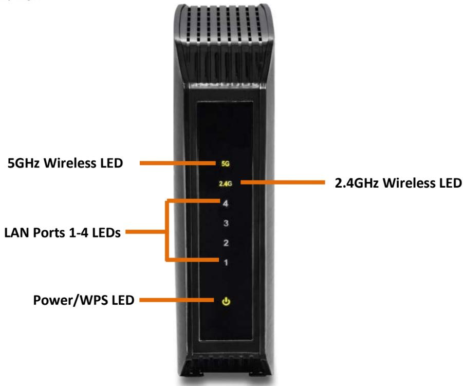
**5G** **5GHz Wireless (Link/Activity) LED:** The indicator will turn solid green when 5GHz wireless is enabled on your media bridge. The indicator will blink when data is transmitted or received from 5GHz wireless devices connected to your media bridge.
