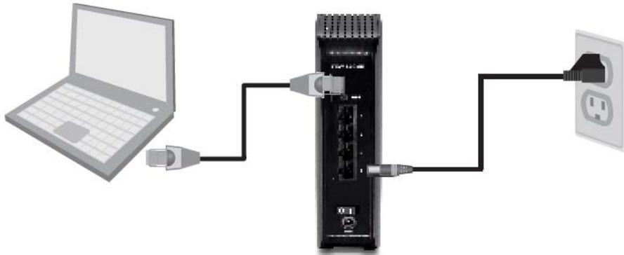
1. As illustrated above, connect one end of the provided RJ-45 network cable to one of the TEW-800MB's network ports. Connect the other end of the cable to your computer's network port\*\*; move on to the next step.
