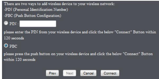
**Note:** You may need to initiate the WPS PIN on your wireless device first when using this method. Refer to your wireless device documentation for details on the operation of WPS.
