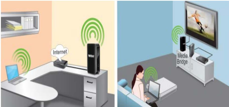
The router is installed near the modem typically supplied by your ISP “Internet Service Provider. The router’s WAN port is physically connected to the modem’s network port which connects to the Internet. Wireless signals from the router are broadcasted to wireless clients such as laptops (with wireless capability) thereby providing Internet access throughout your network.
