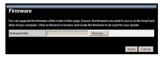
Once you've selected the new firmware file, click **Apply** at the bottom of the screen to start the upgrade process
