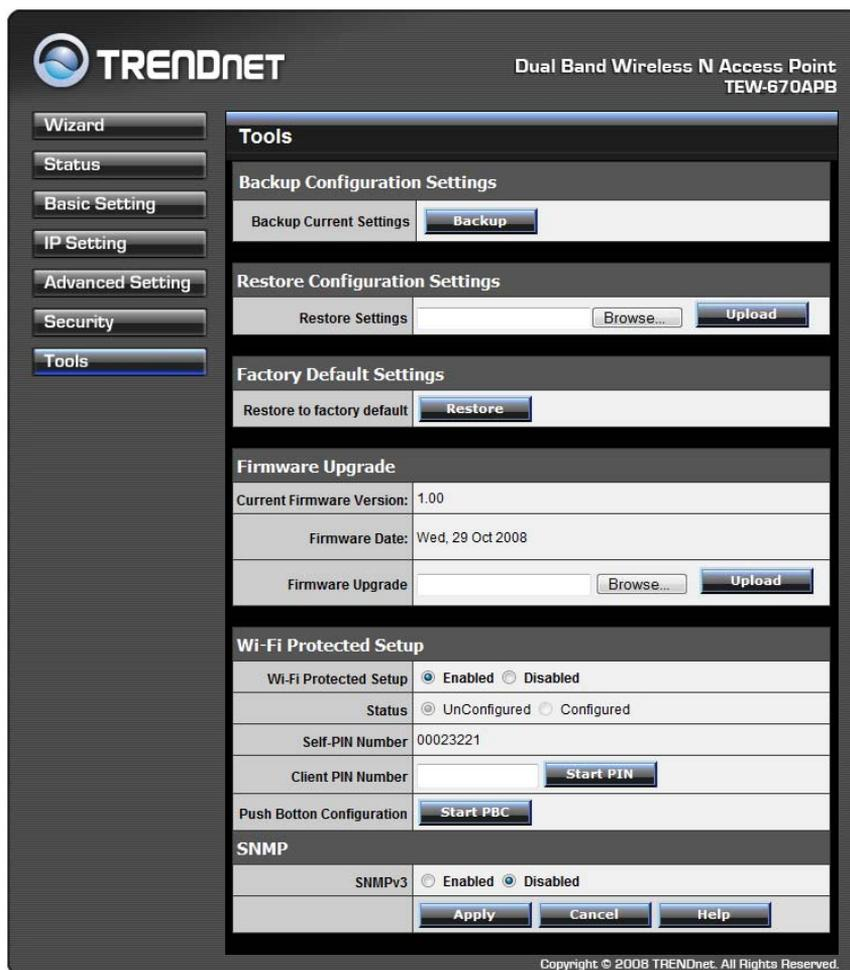
**Backup Current Setting:** Click on “**Backup Current Setting**” button, which will open a FileSave Dialog box, where users can save the current settings and configurations to a file.
