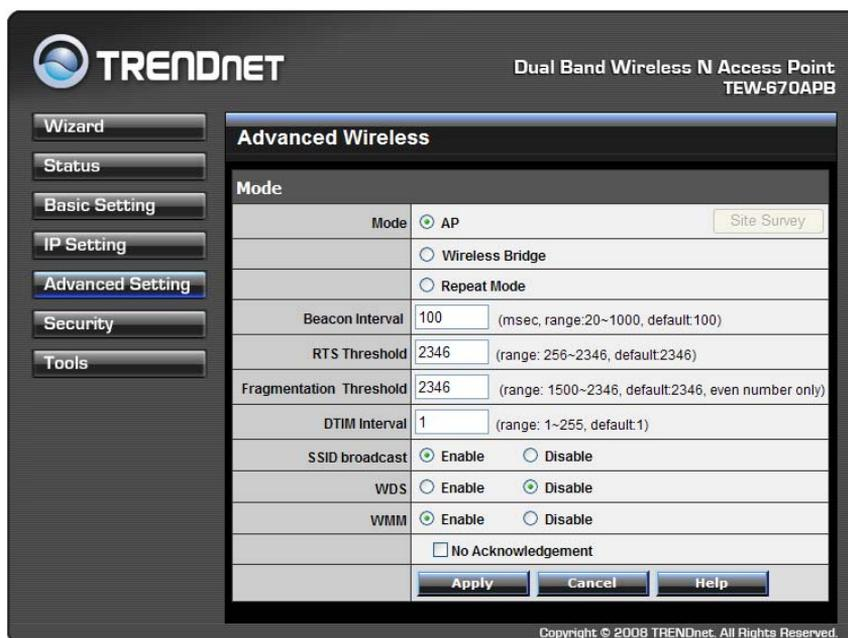
**Mode:** The WLAN AP supports three operation modes for Access Point, Wireless Bridge, Repeater modes.
