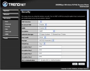
**ESSID Selection:** As this device supports multiple SSIDs, it is possible to configure a different security mode for each SSID (profile). Select an SSID from the drop-down list.
