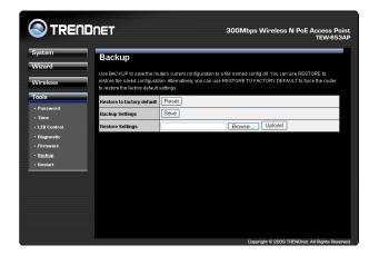
**Backup Settings:** This can save the current configuration to a file named "<u>config.bin</u>" on your PC. You can also use the **Upload** button to restore the saved configuration to the Broadband router. Alternatively, you can use the "**Restore to Factory Defaults**" tool to force the Broadband router to perform a power reset and restore the original factory settings.
