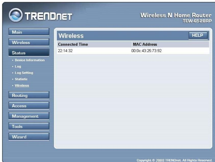
The screenshot shows the TrendNet web interface for a Wireless N Home Router (TEW-652BRP). The left sidebar contains navigation buttons for Main, Wireless, Status, Routing, Access, Management, Tools, and Wizard. The Wireless section is expanded to show Device Information, Log, Log Setting, Statistic, and Wireless. The main content area is titled 'Wireless' and contains a table with the following data:
