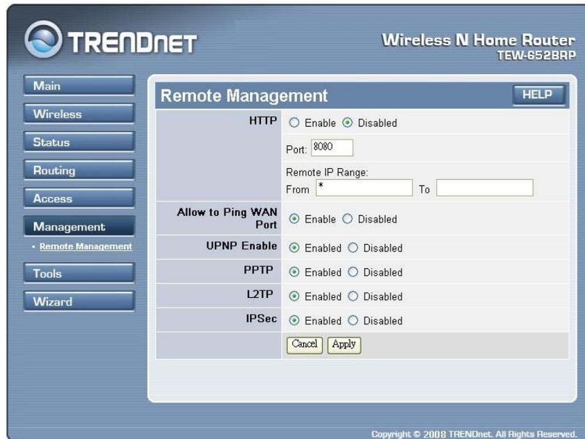
**HTTP:** Enables users to set up HTTP access of the Port number, and Remote IP Range for remote management.
