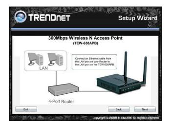
6. Plug in the power adapter of the TEW-638PAP and plug in the device that you will be connecting together. Verify the Power & Ethernet LEDs are light. *EU Version please make sure the power switch is on the On position*
