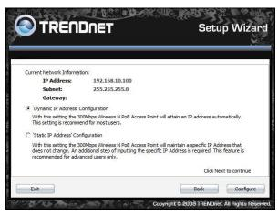
3. The default IP address is 192.168.10.100, you can choose to obtain network setting automatically, or set the IP address manually. After setting, click **Next** to continue.
