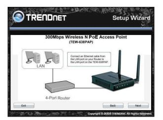
1. Plug in the power adapter of the TEW-638PAP and plug in the device that you will be connecting together. Verify the Power & Ethernet LEDs are light. *EU Version please make sure the power switch is on the On position*
