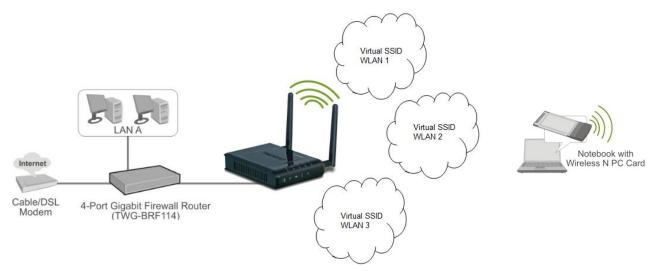
Multiple SSID (Virtual WLANs)
