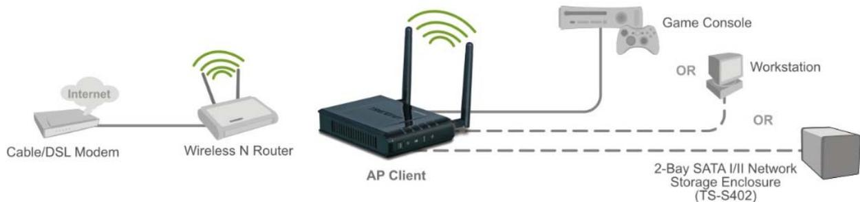
AP Client allows Ethernet enabled devices to become wirelessly enabled.
