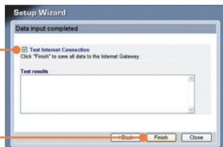
11. Verify that the test has completed successfully. Check that the ADSL and Internet LEDs are lit. Then click **Close**.
