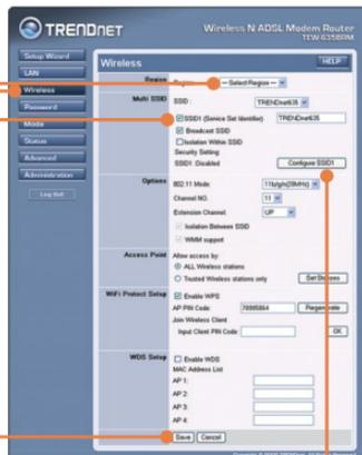
2. Click **Configure SSID1** to set up **Wireless Security**.
