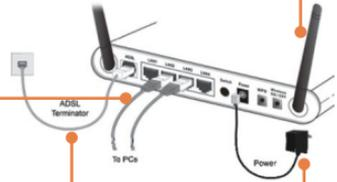
2. Connect one end of the RJ-11 cable to the TEW-635BRM's ADSL port. Connect the other end of the cable to the phone jack.
