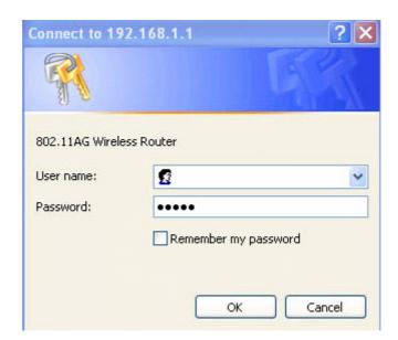
In order to configure the Wireless 11ag Router, you must input the password into the **Password** box and leave blank on the **User Name** box. The default password is "admin".
