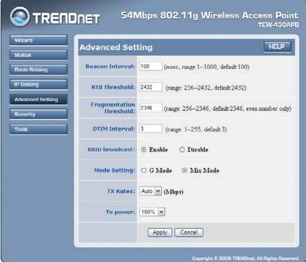
The screenshot displays the 'Advanced Setting' page for a TrendNet 54Mbps 802.11g Wireless Access Point (TEW-430APB). The page is divided into a left sidebar with navigation buttons (Wizard, Status, Basic Setting, IP Setting, Advanced Setting, Security, Tools) and a main content area. The main content area contains the following settings:
