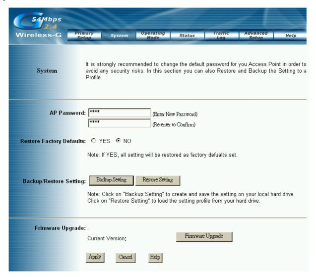
**AP Password:** Changing the password for the AP is as easy as typing the password into the **Enter New Password** field. Then, type it again into the Re-enter to confirm.
