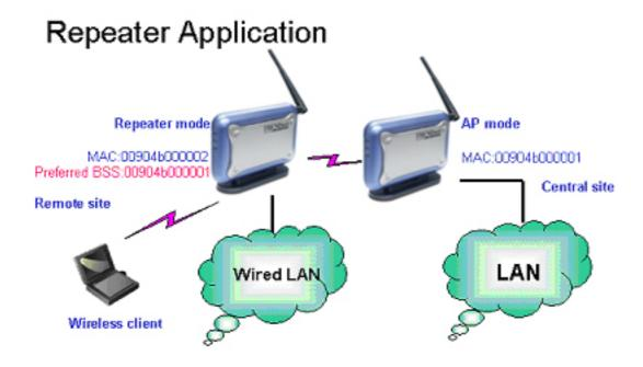
Wireless Bridge: This mode allows the connection of one or more remote LANs with a central LAN.
