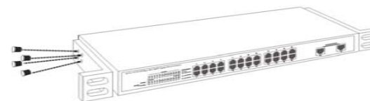
Figure 1. Combine the Switch with the provided screws
