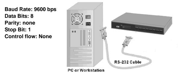
Figure 4-1. The settings of communication parameters
