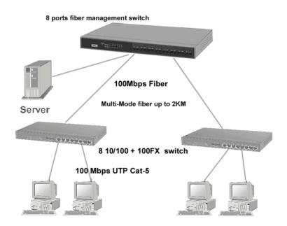
Figure 3-3 Use fiber port (TEG-S081Fi Switch) to extend the distance between workgroups
