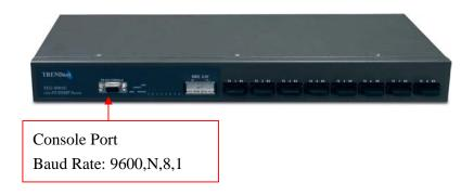
Figure 2-2. The Front Panel of the TEG-S081Fi Switch with SC connector
