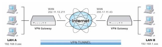
Figure 56: Connecting 2 TW100-BRV204 s
