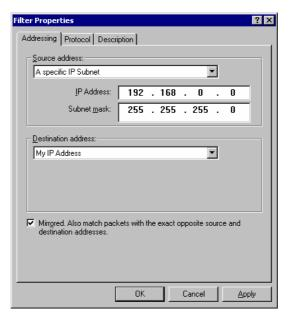
Figure 71: Filter Properties: Addressing
