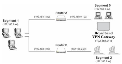
Figure 117: Routing Example
