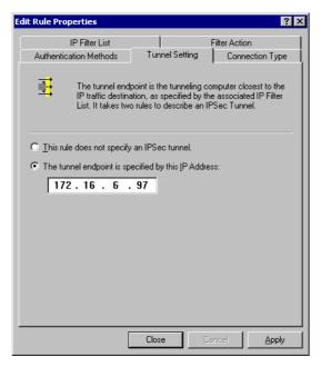
Figure 67: Tunnel Setting
