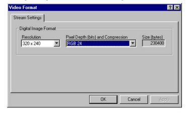
Note: The higher the RGB bits, the larger the video file size well be. The lower resolution is recommended for video-conferencing or recording video. after this step the Configuration Advisor will check to ensure that the installation went smoothly.
