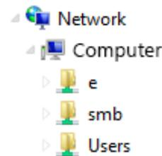
**Tip:** To create a network storage on your Windows® based system, create a shared folder and then test your set up with another computer. Enter the IP address of the computer here and enter the shared folder name with a leading forward slash. For example, if you have a shared folder named "SMB", enter "/SMB" in the **File Path**.
