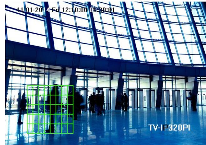
**Draw Area:** Click **Draw Area** button to start drawing. Click and drag on the area you want to set up the motion detection. You can draw up to 8 different areas. Click **Stop Drawing** to stop drawing motion detection areas.
