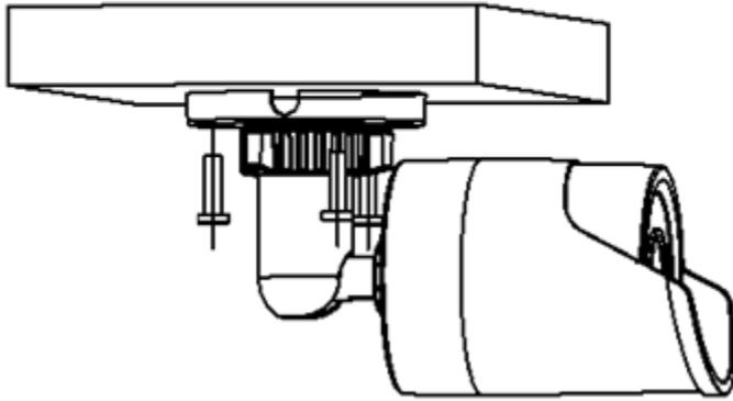
Loosen the lock ring and then adjust the camera position. Tighten the lock ring when you setup the camera position.
