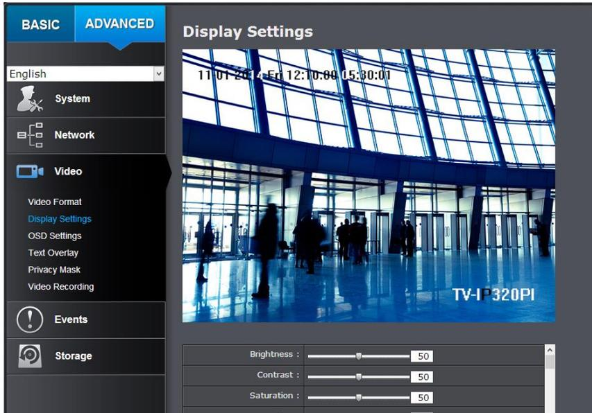
**Brightness:** Use the slider or enter a number (0-100) to adjust the image brightness. Default: 50
