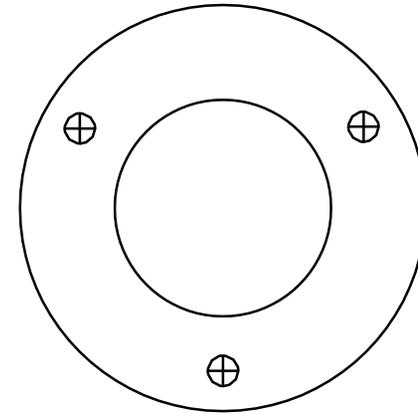
Fix the mounting base on the ceiling or the wall with the screws that come with the package. Route the cables to the cable hole.
