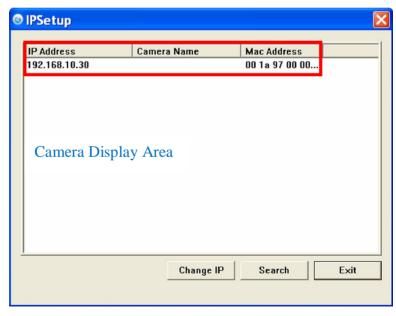
**Camera Display Area:** It shows the connected camera(s) within the same network.
