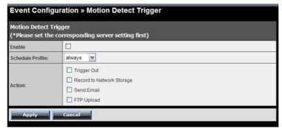
Schedule Profile: Select the Enable option to enable the trigger function of the camera, so that you can send captured images within the detecting area to the FTP server, email receiver, Network Storage server, or the connected USB device. You have to configure corresponding settings, such as FTP server and email server, to enable this feature. Please note that you have to configure the related settings before enabling these features
