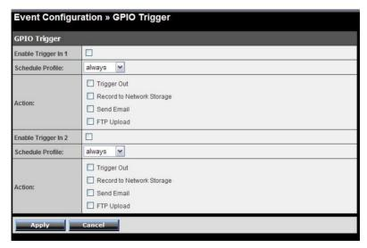
The GPIO trigger function of the camera allows you to set Trigger Out function or send captured images within the detecting area to the Network Storage server, email receiver, or FTP server. You have to configure corresponding settings, such as FTP server and email server, to enable this feature.
