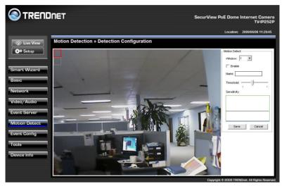
To enable the detecting area, select **Window 1** or **2** from the pull-down list, and then select **Enable**. When the detecting area is enabled, you can use the mouse to move the detecting area and change the area coverage.
