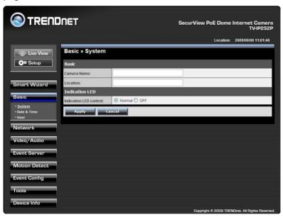
The Web Configuration contains the settings that are required for the camera in the left menu bar, including **Smart Wizard**, **Basic**, **Network**, **Video/Audio**, **Event Server**, **Motion detect**, **Event Config**, **Tools**, **USB**, and **Information**.
