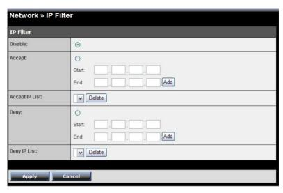
The IP Filter setting allows the administrator to limit the users within a certain range of IP addresses to have access to the camera.
