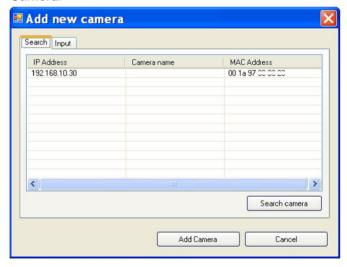
Select the Input tab to add a camera by entering its IP Address directly. Enter the camera's IP Address (default: 192.168.10.30) and Port (default: 80), and then click Add Camera.
