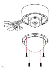
2. Drill three pilot holes into the ceiling and hammer the plastic anchors into the holes.
