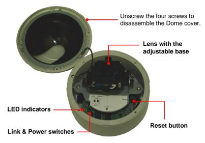
Reset button: Press the button to restart the camera.
