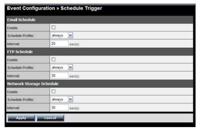
You can separately configure the schedule for trigger function of the camera by **Email**, **FTP**, or **Network Storage**. Select
