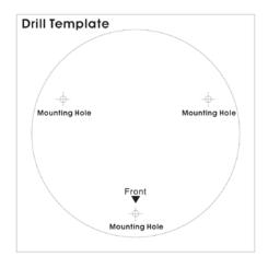
3. Install the camera to the ceiling with three screws.
