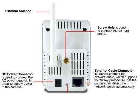
Reset Button will restart the camera when it is pressed quickly; when it is long pressed for five seconds, the camera will resume the factory default settings.
