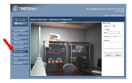
To enable the detecting area, select **Window 1** or **2** from the pulldown list, and then select **Enable**. When the detecting area is enabled, you can use the mouse to move the detecting area and change the area coverage.
