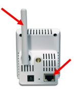
Attach the external power supply to the DC power input connector located on Camera's real Panel, and then connect it to your local power supply.
