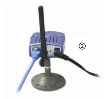
**TIP:** You can confirm power source is supplied from the LED indicators label Power on the Wireless Internet Camera is illuminated.
