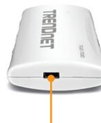
Connessione al computer mediante USB 2,0
