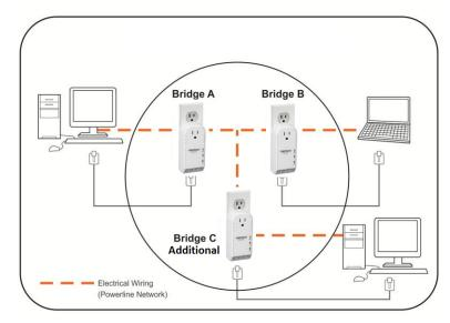
Assuming the two TPL-307E powerline adapters are currently connected to each other and the third TPL-307E (Additional) powerline adapter is currently disconnected.
