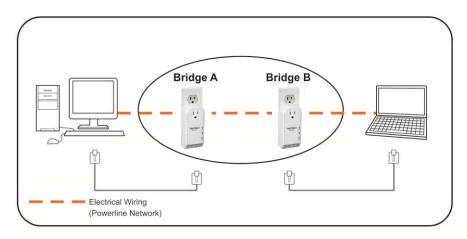
Assuming your TPL-307E powerline adapters are already plugged into wall power outlets and either currently connected or disconnected to each other.
