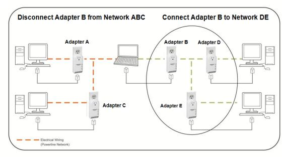
Assuming all powerline adapters are TPL-307E adapters and for reference in the diagram and this procedure, the adapters will be labeled *Adapter A, B, C, D,* and *E. Adapters A, B,* and *C* are currently connect together to form one powerline network and *Adapters D* and *E* form another powerline network. *Adapter B* will be disconnected from *Adapters A* and *C* and connected to *Adapters D* and *E*.
