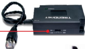
2. Connect an Ethernet cable from a PoE port on the TPE-S80 switch to the **PoE IN** port on the TPE-112GS.
