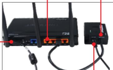
4. Connect the provided Jumper cable to the non-PoE device (e.g. TEW-639GR) and to the TPE-112GS.
