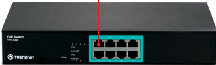
4. Connect a RJ-45 cable from a PoE port (1~8) on the TPE-S80 to the **LAN** port of the PoE device (e.g. TEW-638PAP)
