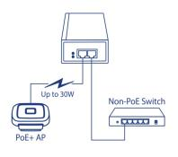
**PoE+** The 2.5G PoE+ injector supplies a PoE device with PoE (15.4W) or PoE+ (30W) power.
