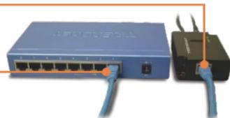
3. Connect the Ethernet cable from the **Data-Out** port on the TPE-102S to the non-PoE device's LAN port (e.g. TEW-450APB).
