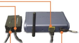
4. Connect the provided Jumper cable to a non-PoE device (e.g. TEW-450APB) and to the TPE-102S.
