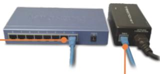
3. Connect a CAT-5 cable from a PoE device (e.g. TEW-434APB) to the TPE-101I's **PoE Out** port
