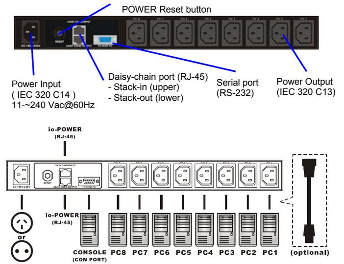
You might need to use extra adapter cords between TK-RP08 and your devices, especially when the devices are not of the plug specification that fits the standard power outlets on the back panel of TK-RP08. These adapter chords are not included with your package carton and are available by optional purchase.
