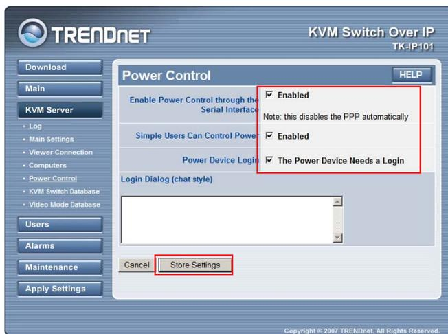
Once the *Enabled* option is checked, a subsequent Power Device Login option will appear for you to decide whether to enter the login script. The TK-RP08 does not require a login script. Hence you don't have to enter any script.
