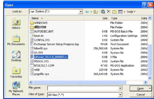
Then select the correct firmware upgrade file, e.g. TK-RP08\_V.x.x.x\_dddxxx Then click *Open* to start firmware upgrade.
