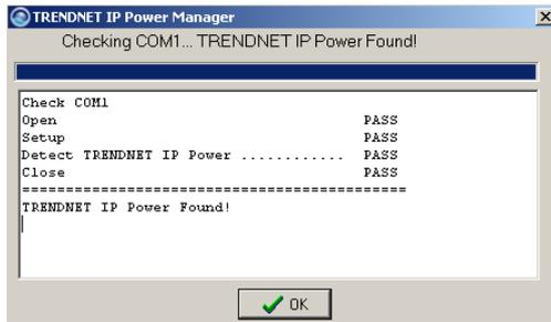
Check the COM port detection message on the message Box. After the COM port has been successfully detected, click *OK* to connect.
