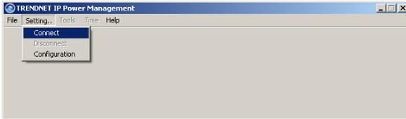
**Step 2.** Connect the host PC to TK-RP08 by clicking *Setting/Connect*. And the software will automatically detect COM port for TK-RP08 ....
