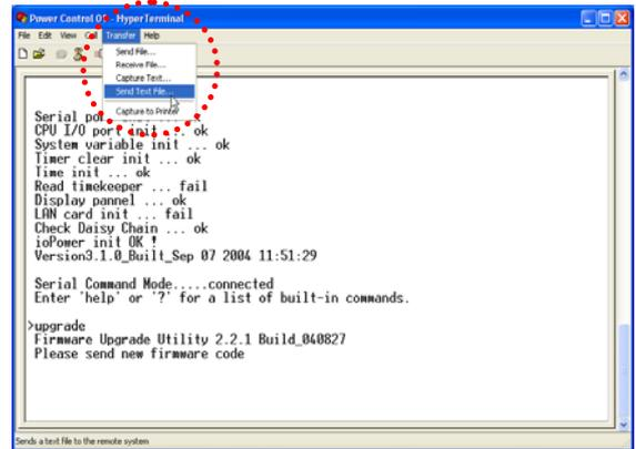
....and a dialog box will prompt you to select the flash upgrade file, \*.x (with a file extension name as .x). In this case, we have our flash upgrade file as *TK-RP08 3.0.1\_040907.x* (it could be any other file name with an .x extension!). Note that since it has an extension name other than .txt, we have to select the "All file [\*.\*]" option in order to see it on the file listing....
