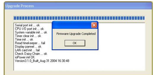
You can also use the Windows HyperTerminal to perform firmware upgrade, please refer to the *Firmware Upgrade Operation Guide* that comes with your firmware upgrade file. Normally, your TK-RP08 unit is loaded with the latest firmware, you should have no need to reload/upgrade your firmware unless (1) there's a new firmware upgrade ready (2) your firmware is corrupted and need reloading.
