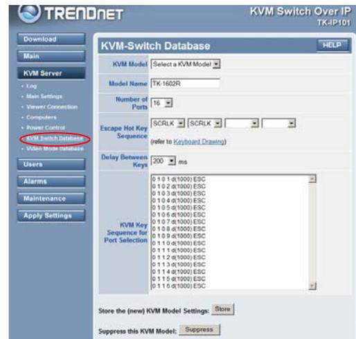
The various settings on this page are KVM port-specific because a computer is first identified by the KVM port it is attached to. Select the target port on which your subsequent settings on this page are directed. You can use the drop-down combo box as well as use the *Previous* and the *Next* button to navigate to a specific port.
