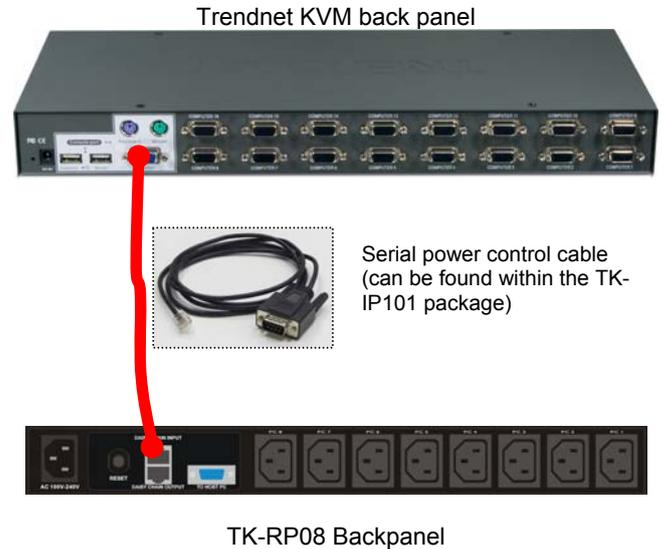
**Step 2.** Make sure that the TK-IP101 and TK-RP08 are powered on. If not, power them up first before proceeding.
