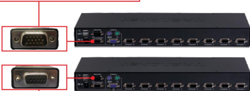
2. Connect the opposite end of the daisy-chain cable to the **Daisy-Chain IN** port on the second (slave) KVM switch.
