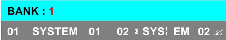
After selecting the desired PC Name, press “ INS” key to edit PC name. The name can be up to 10 characters long (please use only numbers and/or letters). After finishing the name edit, press “Enter “ key to save the information.
