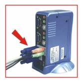
**3.** Connect each set of integrated KVM cables to each computer's video, PS/2, mouse, USB, speakers, and microphone connectors.
