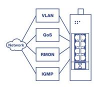
Integration Flexibility Managed layer 2 features include VLAN, IGMP snooping, QoS, RMON, SNMP trap, and syslog for monitoring and flexible network integration.
