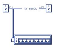
**Redundant Power** The industrial Ethernet switches feature dual power inputs to provide redundant power with overload current protection.
