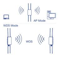
Wireless Modes Supports Access Point, WDS Bridge, WDS Access Point, WDS Station, and Client Bridge modes for a variety of wireless applications.
