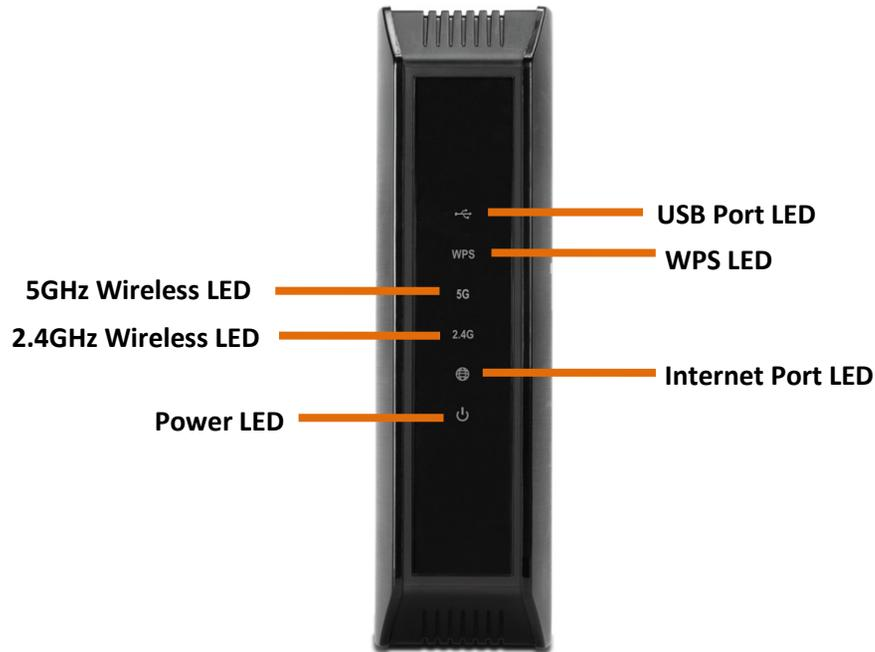
**USB LED:** The LED will turn on when a USB storage device is connected to the USB 2.0 port.
