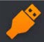
**USB:** The USB icon displays orange to indicate that there are no USB devices connect to the USB port(s). The USB icon displays green to indicate that are USB devices connected to the USB port(s).
