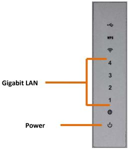
8. Verify that the following front panel LED indicators on your router: Power (Solid Green), Gigabit LAN 1, 2, 3, or 4 (Solid/Blinking Green for ports for which devices are connected), WAN (Solid/Blinking Green).
