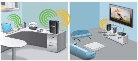
The router's gigabit Internet port is connected to your Internet modem which is connected to the Internet. Wireless signals from the router are broadcasted to wireless clients such as laptops (with wireless capability), TVs or media bridges thereby providing Internet access.
