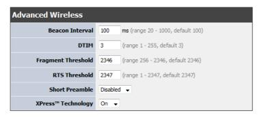
• **Beacon Interval:** A beacon is a management frame used in wireless networks that transmitted periodically to announce the presence and provide information about the router's wireless network. The interval is the amount time between each beacon transmission.
