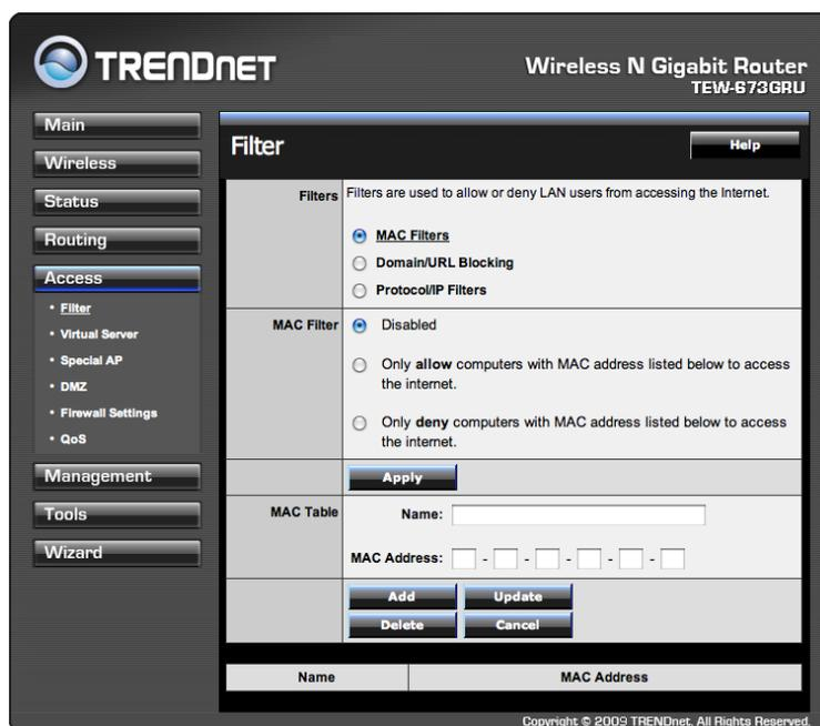
**MAC Filter:** Enables you to allow or deny network access to LAN and/or WLAN users based upon the MAC address of their network interface.
