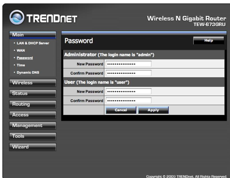
**Administrator:** Type the password the Administrator will use to log into the system. The password must be typed again for confirmation. The Administrator have the ability to apply and setting on the WLAN Router.
