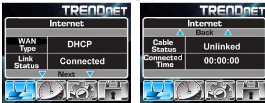
3. To go back to the Device Info menu or the Main Menu screen, press ▲ repeatedly until the desired menu or screen is reached.
