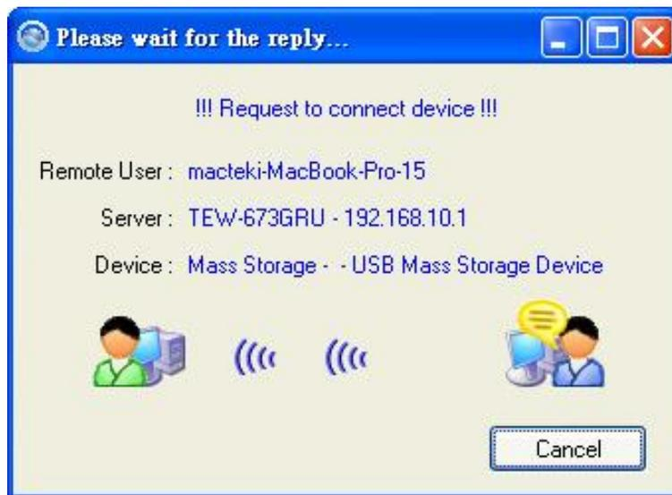
Note: Only a single user can establish connection to a USB device. Once the “Request to Connect” is approved, the connection to the USB device will automatically transfer to the requested user.
