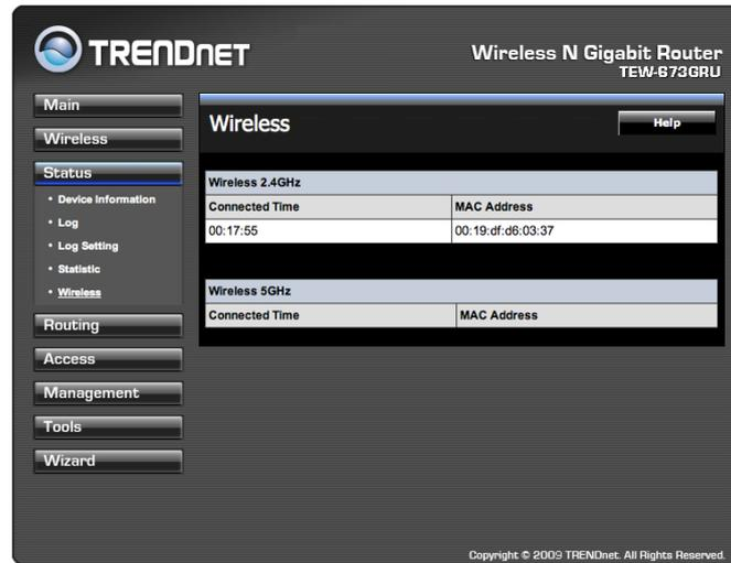
**Connected Time:** Lists all wireless clients and how long they have been connected WLAN Router.
