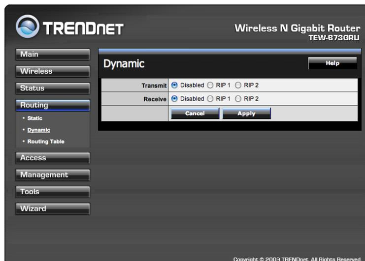
**Transmit:** Click the radio buttons to set the desired transmit parameters, Disabled, RIP 1, or RIP 2.
