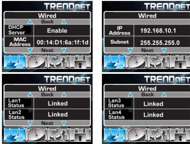
3. To go back to the Device Info menu or the Main Menu screen, press ▲ repeatedly until the desired menu or screen is reached.
