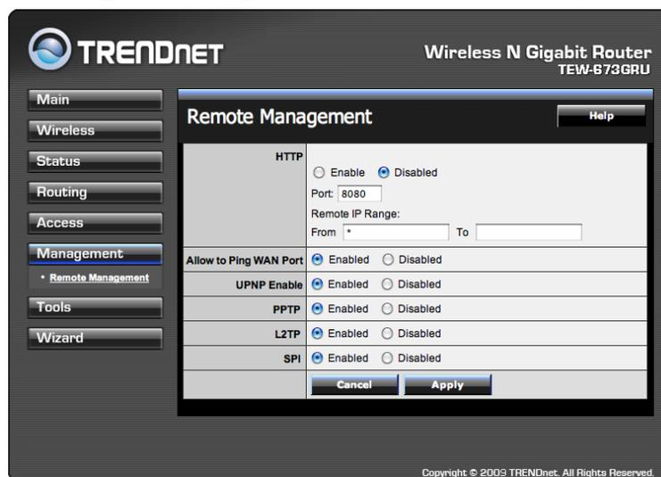
**HTTP:** Enables users to set up HTTP access for remote management.
