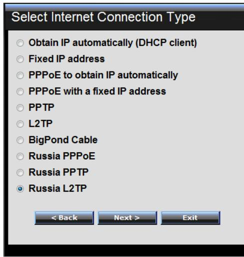
If connected to the Internet using Russian L2TP (Dial-up xDSL) enter your server IP, PPTP Account and Password. If using Static IP you must enter your IP, Subnet Mask, Gateway, Server IP, PPTP Account and PPTP Password.
