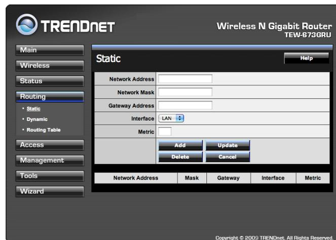
**Network Address:** Type the static IP address the network uses to access the Internet. Contact the ISP or network administrator for this information.
